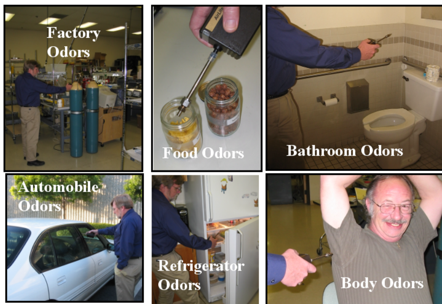
Figure 2- Battery operated remote sampler can be used to collect vapors from many different types of odors.
