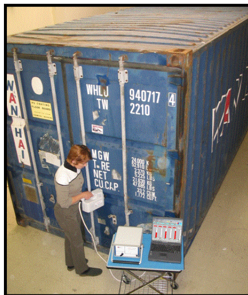
Figure 3- Vapors are sampled by inserting a probe attached to the inlet of the instrument into a small re-sealable hole in the container.
