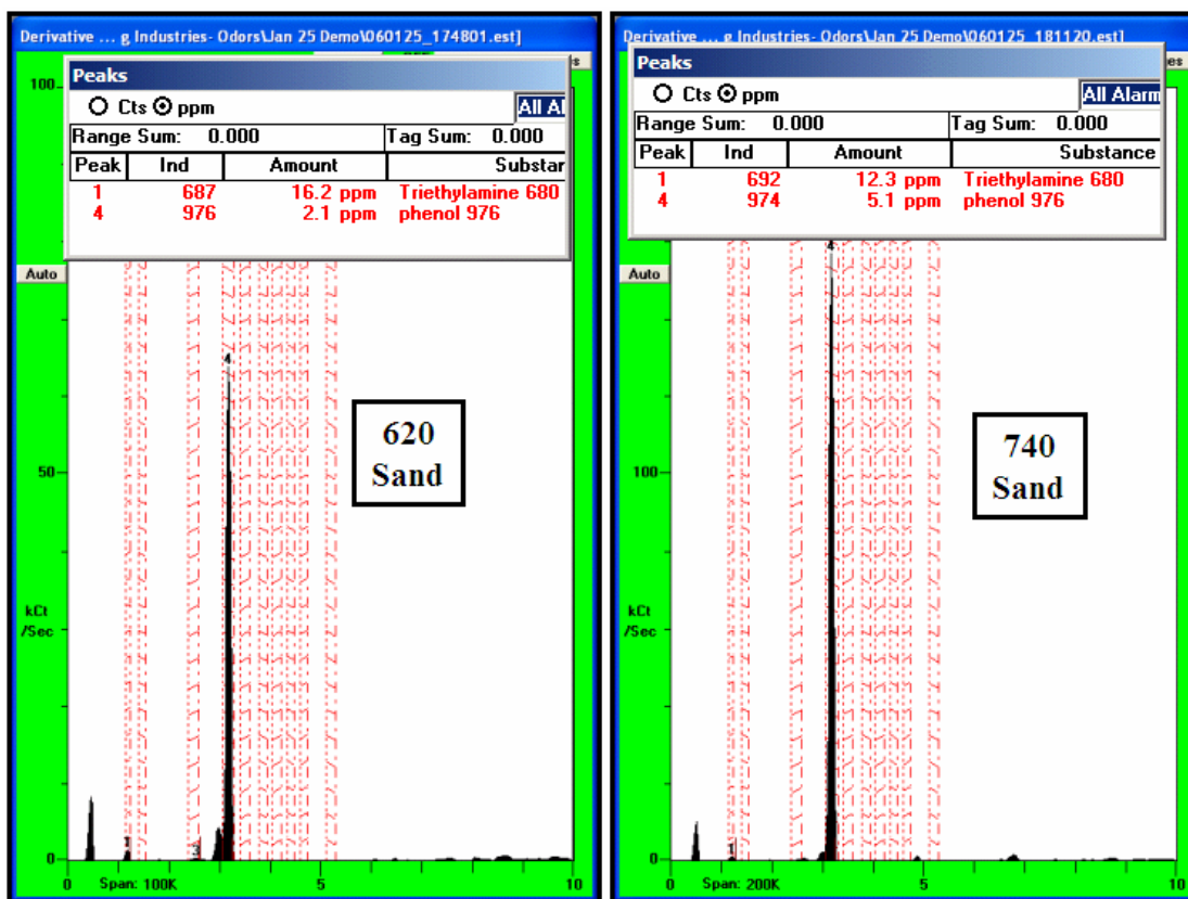
Figure 16- Odors from sand samples in septa sealed vials. Note different vertical scales of 100 and 200 kcts/sec are used to display chromatogram results.
