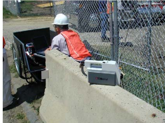
Figure 17- Real time monitoring of site odors located at street entrance (downwind).
