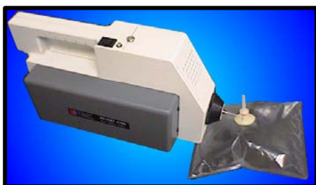
Figure 13- Tedlar bags make constant concentration vapor standards for calibration of the zNose™.
