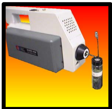
Figure 11- Calibrating with standard vapor concentration.
